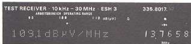
Fig. 15 Front-panel frequency display and alphanumeric display for readout of measured data, input and output of setting data and output of error messages.
