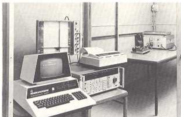
Fig. 4 Automatic measurement of interference voltage with programmed phase switchover (Test Receiver ESH 3, Printer PUD, XY Recorder ZSKT, Artificial Mains Network (LISN) ESH 2-Z5, Process Controller PPC, and Code Converter PCW). Door to test item open for demonstration purposes.
